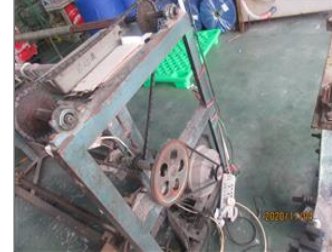
Photo of non-conformity NC - 7.17 No safeguards were installed on transmission belt.JPG
