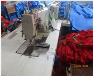
Photo of non-conformity NC - 7.17 sewing machines in the sewing workshop were not equipped with needle guard.JPG
