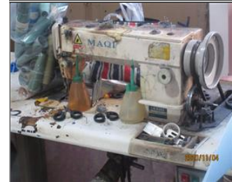
Photo of non-conformity NC - 7.7 No label was attached for the machine oil container.JPG
